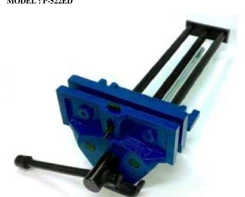
Manufactured with a close grained cast iron body and steel lead screw. The quick release mechanism is engaged using a trigger action. Clamping control is returned to the screw upon release of the trigger. Designed for bench mounting. Fitted with a front dog, which when used in conjunction with a bench stop, allows oversize work to be held secure.
